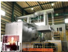
High frequency induction furnace The furnace for experiments or melting on contract. All kinds of analysis are available on the spot.
